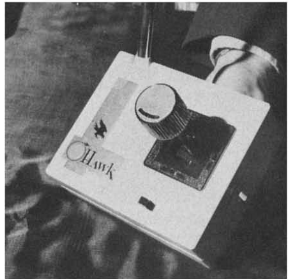
Orbit Electronics , (1641 Kaiser Ave., Santa Ana, CA 92705) was proudly hawking their new "Hawk" 3-4 channel radio with 6 interchangeable frequency crystals for 27MHz band. Dry cell or rechargeable transmitter power supply. Flying weight with two servos is 9-oz. Under $200.
